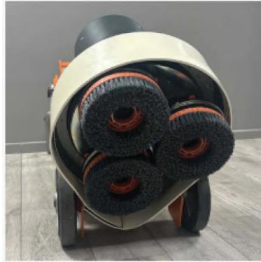
Gear Plate with Aging Brushes
