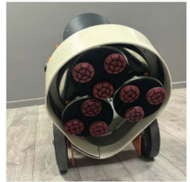
Resin bond tools for granite
